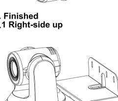
3.Slide the tray with the PTZ camera fixed to it into the grooves of the L-shaped stand. Then tighten the screws on both sides.
