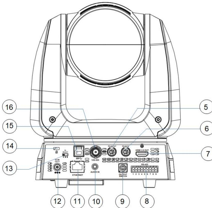
**<Remark> The figure is an example of VC-A71P. VC-A71PN does not support SDI and USB output.**
