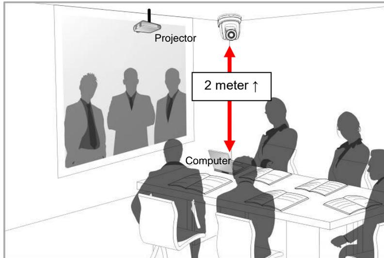
3. The machine (including metal plates) is weighed at about **3 kg**. If it is to be installed on the ceiling, please use the hanger that has obtained UL security approval to prevent the machine from falling down.
