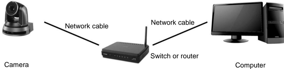
2. To connect directly through network cable, the IP address of the computer should be changed so that it is on the same network segment as the camera
