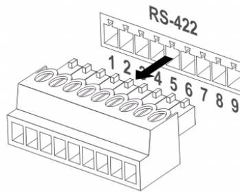
2. Peel off a section of copper wire (AWG Nos. 28 to 18) and insert it into the connector hole; then use flat screw driver to fix it
