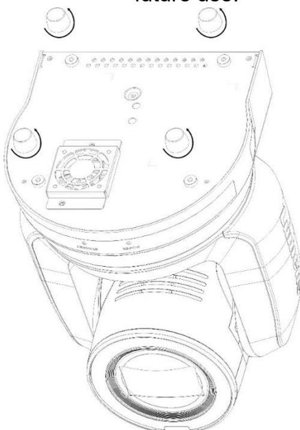
2. Fix the metal plate A on the machine base with 4 M3 silver screws
