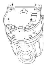
3.Lock the metal plate B on ceiling mounted
