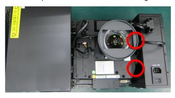
2.2.2. Make sure connection cables are connected, two cables in total
