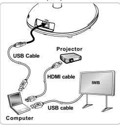
Once the USB is connected to the computer, the power is ON. When the LED signal lights RED, the image is on display.
