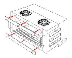
**Note:** The thumbscrews are connected to the locking panels with a retentionmechanism and will not come completely free when they have been unscrewed from the chassis.
