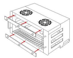
**Note:** Be careful to not overtighten the thumbscrews as this could damage the screw threads.
